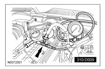
10. **NOTE:** The Fuel Pump Driver Module (FPDM) was previously disconnected in the Fuel System Pressure Release and must be reconnected to complete the Fuel System Pressure Test.
